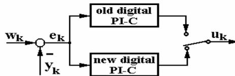
Figure 8. Transfer from the old digital PI-C to the new one
